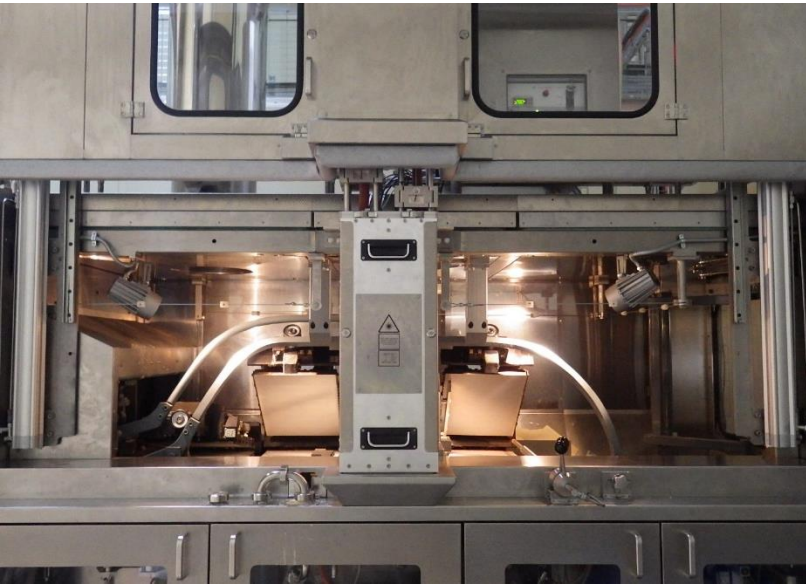
Flat wafer oven with large plate and small opening angle
