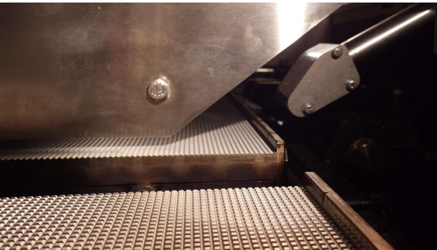
bakeLINE optics cleaning a wafer oven during operation
