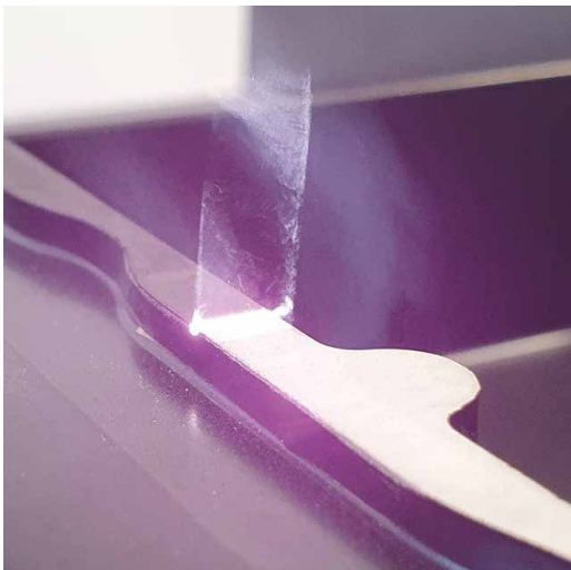
cleanLASER in the production of battery housings
