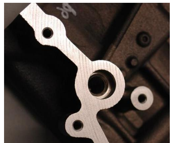
Sealing contour with preserved milling structure after laser processing
