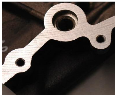
Sealing contour with preserved milled structure after laser treatment
