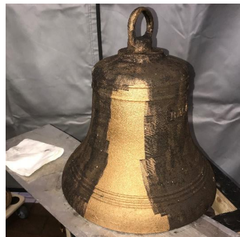
The CleanLASER allows, for example, the removal of substance-damaging salt deposits and corrosion without destroying the naturally evolved protective passivation of bronze or other metals. (Photos: Wolfmeyer zu Barkholz)
