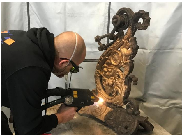
The CleanLASER allows, for example, the removal of substance-damaging salt deposits and corrosion without destroying the naturally evolved protective passivation of bronze or other metals. (Photos: Wolfmeyer zu Barkholz)
