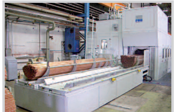
Special facility for cleaning of pipes up to 6 m long
