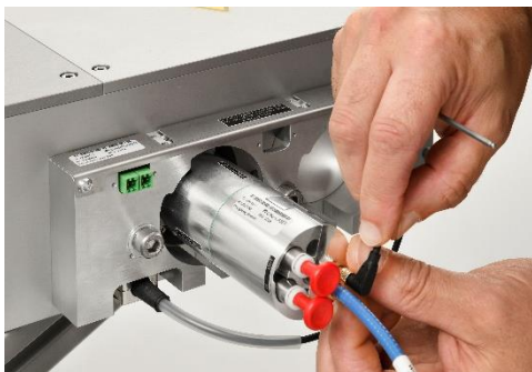
Plugging in the temperature sensor ...
