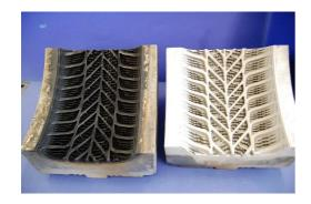
The laser cleans the sensitive mold surface damage- and residue-free, even applied to valves for mold venting such as "Eurovents" or "Thielmannvents". Due to the absence of mechanical force, profile ridges remain undeformed. The process thus extends the service life of the molds and the quality of the tires at the same time. The same applies to "puzzle molds", as their edges are particularly well protected by laser processing.
