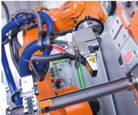
cleanLASER during welding pre-treatment in body-in-white production
