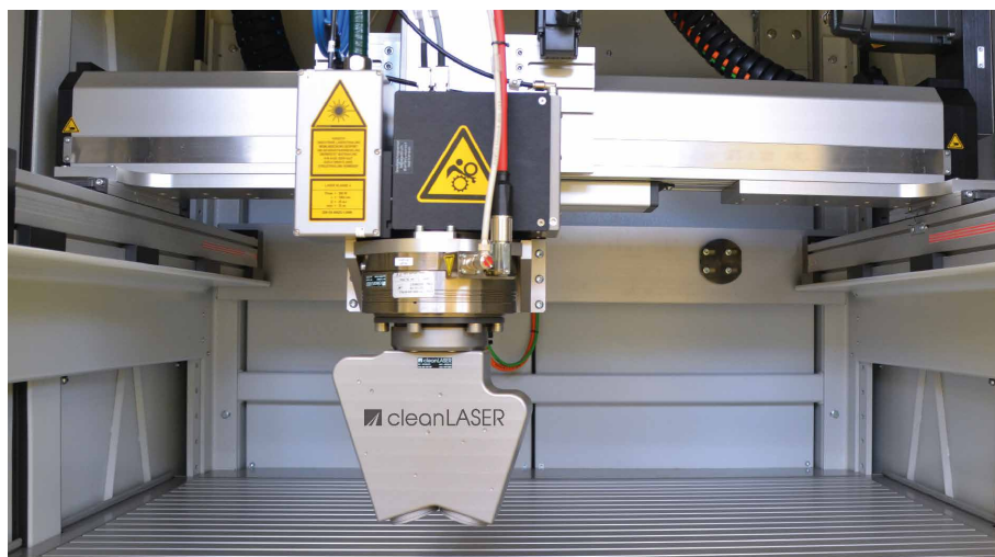
cleanCELL-Portal with shareMOTION optic for efficient adhesive pre-treatment
