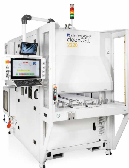
cleanCELL 2220 with double-drawer module for the processing of control units
