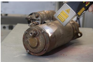
The cleanDECONT can be used in an economically and eco-friendly way for decontamination in nuclear areas. As a dry process, laser light replaces the chemical wet process and the mechanical blasting.
