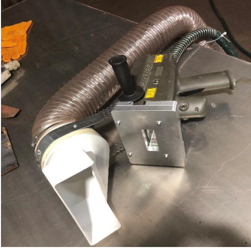
CL 1000 with suction nozzle and contamination cover plate
