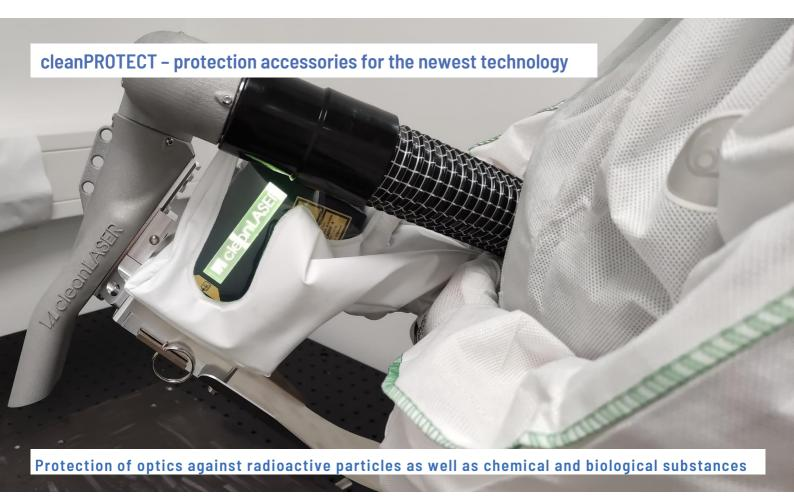
The use of the laser in areas with toxic and radiological contamination requires the protection of the optics and the optic fiber along with personnel protection provided by selected suits, masks and gloves. The protective cover can be decontaminated or cleaned to prevent cross-decontamination. In case of heavy contamination, the cover can be disposed of or burned according to established practices.
