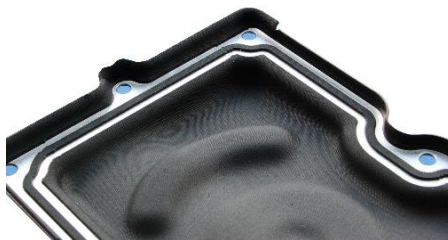
Sealing pre-treatment of an aluminum housing
